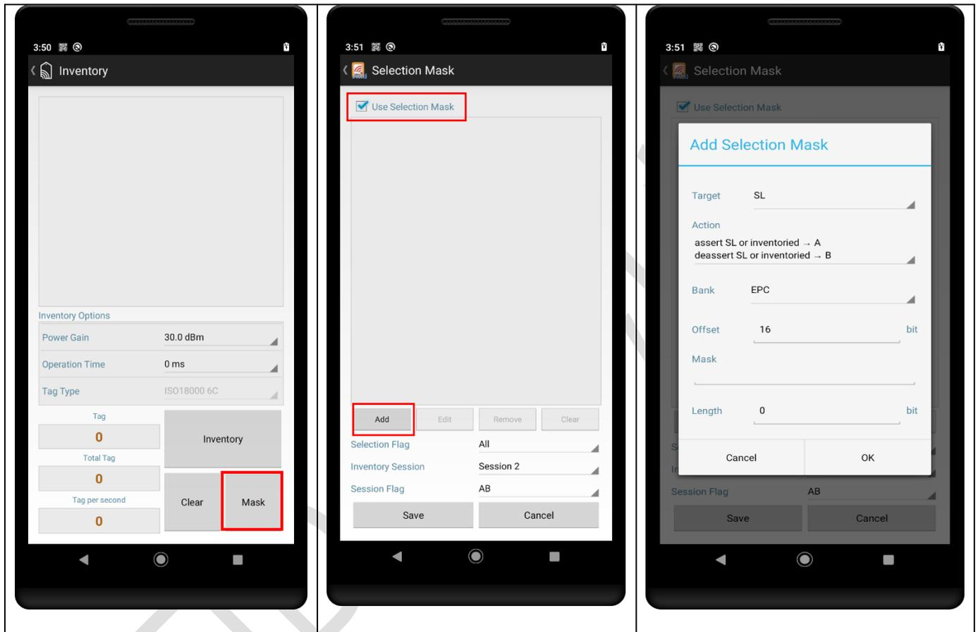
Selection Mask is to set conditions according to Inventory or Access functions, consist of Selection Mask List, conditions to set according to tag, Selection Option, and menu button to set.
