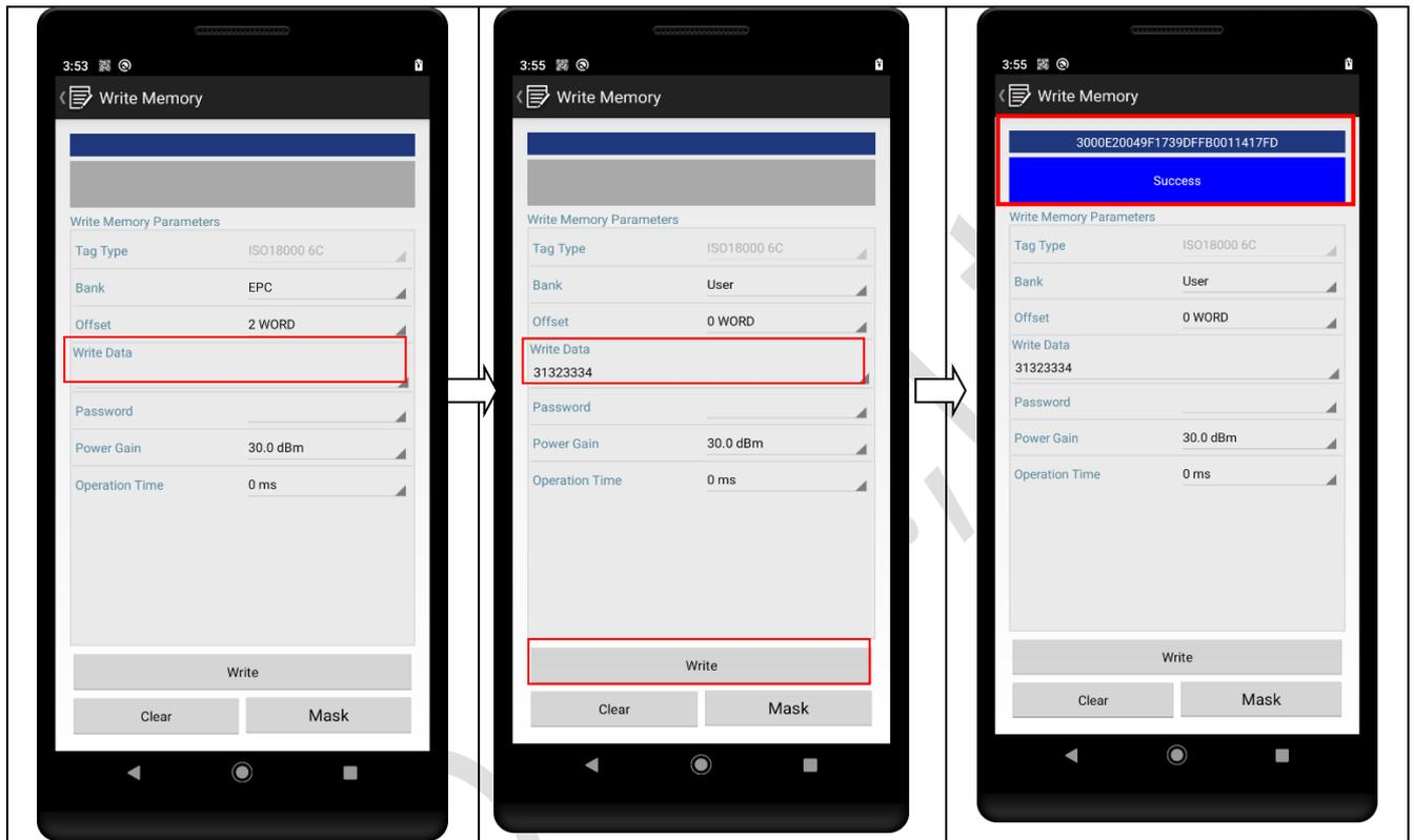
Write Memory screen is consisted of Write Memory Value (displays the results), Write Memory Parameters (sets the parameter values), and Menu buttons.
