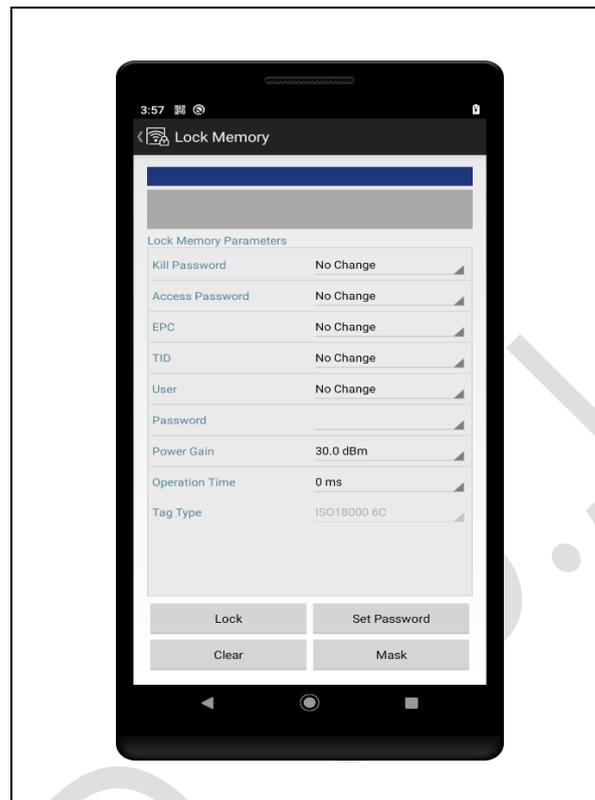
Lock Memory screen is consisted of Lock Memory Value (displays the results), Lock Memory Parameters (sets the parameter values), and Menu buttons.
